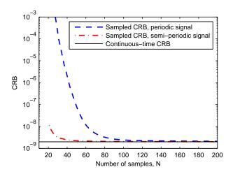
Fig. 5. Comparison between the CRB for a periodic signal (16) and a semiperiodic signal (17).
