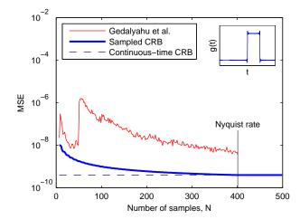
(c) The pulse g(t) is a filtered  $rect(\cdot)$  with 401 Fourier coefficients.
