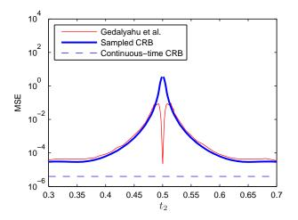
Fig. 3. Comparison between the CRB and the performance of a practical estimator as a function of the pulse positions. The signal contains L=2 pulses, the first of which is located at  $t_1=0.5$ . The MSE is plotted as a function of the position of the second pulse.
